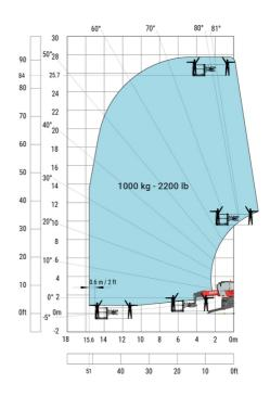
Machine on lowered stabilisers with 3D positive Metric Machine on lowered stabilisers with 3D positive / negative
